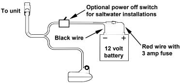
Power and transducer connections for sonar units (direct battery connection shown).
